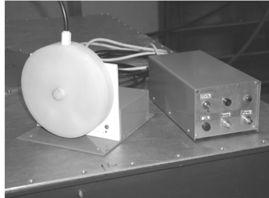
**Figure 9.** The thyristor trigger generator consisting of 2 blocks.
