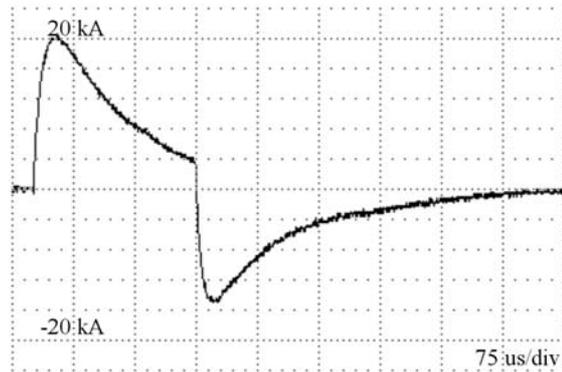
**Figure 5.** Current trace in the preionization circuit at 24 kV charge, 4 C charge transfer.
