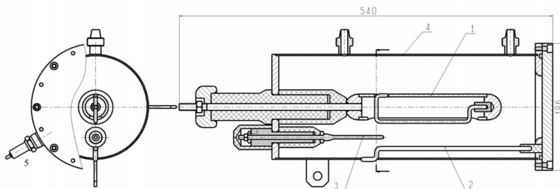
**Figure 4.** Design of the preionization switch.
