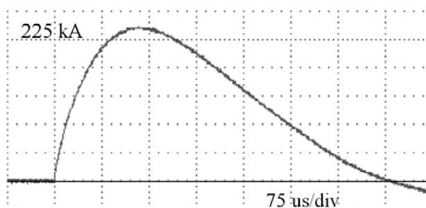
**Figure 7.** Typical current trace in the main switch at 24 kV charge voltage and 70 C charge transfer.
