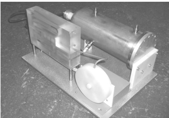
**Figure 3.** The preionization switch.
