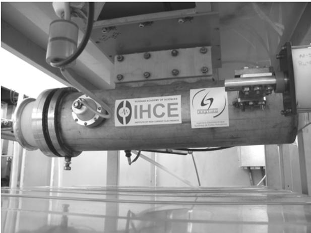
**Figure 8.** The main switch in the capacitor bank.
