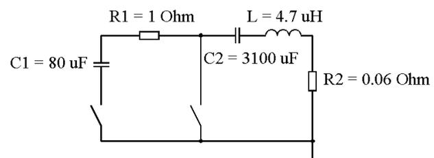
**Figure 1.** Schematics of the test bed circuit with the main and preionization capacitors connected to the load.
