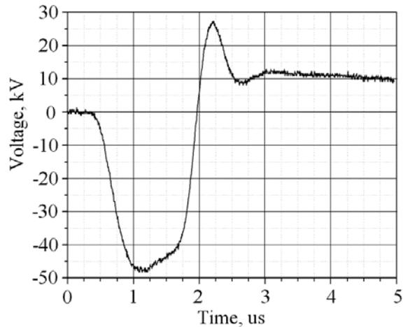
**Figure 10.** Output pulse of the thyristor trigger generator.
