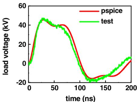
FIG. 15. Recorded and simulated load voltage at  $s = m = 2$ ,  $R_L \sim 1.6$  Ohms, and  $U_{CH} = \pm 100$  kV. The increase of the inductance of the modified bricks causes the top of the pulse to decrease much faster (compare with the traces in Fig. 13).
