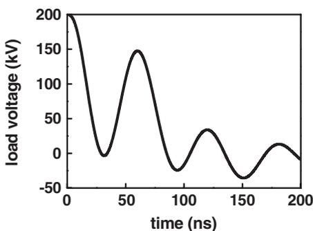
FIG. 9. Simulated voltage across the capacitors in the modified bricks. Same shot as in Fig. 8.
