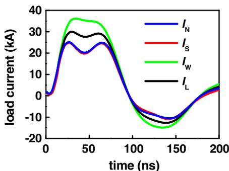
FIG. 14. Load current measured by separate  $B$ -dot probes, and total load current  $I_L$  calculated by using Eq. (11). Same shot as in Fig. 13.
