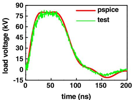
FIG. 8. The recorded and simulated load voltage in a shot without of the current loop around the core, at  $s = 4$ ,  $m = 2$ ,  $R_L \sim 1.6$  Ohms, and  $U_{CH} = \pm 100$  kV.
