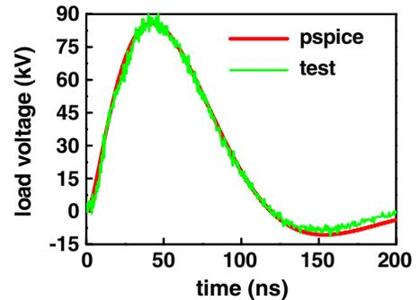
FIG. 7. The recorded and simulated load voltage in a shot without the current loop around the core and without the modified bricks, at  $s = 4$ ,  $m = 0$ ,  $R_L \sim 1.6$  Ohms, and  $U_{\text{CH}} = \pm 100$  kV. The currents  $I_W$ ,  $I_N$ , and  $I_S$  recorded in shots without the modified bricks at each given  $R_L$  were equal within  $\pm 5\%$ .
