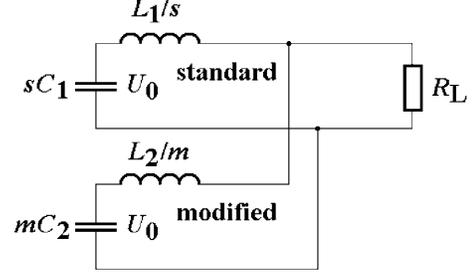
FIG. 3. Simplified electrical circuit of the square pulse LTD.
