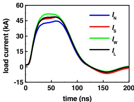
FIG. 10. Load current measured by separate  $B$ -dot probes, and total load current  $I_L$  calculated by using Eq. (11). Same shot as in Fig. 8.
