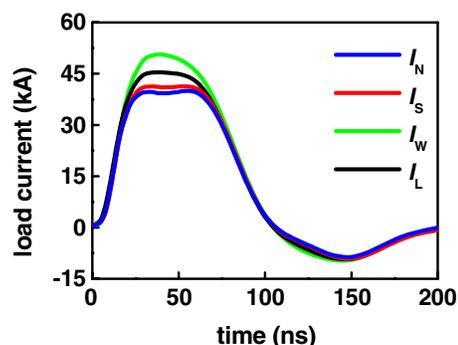
FIG. 12. Load current measured by separate  $B$ -dot probes, and total load current  $I_L$  calculated by using Eq. (11). Same shot as in Fig. 11.
