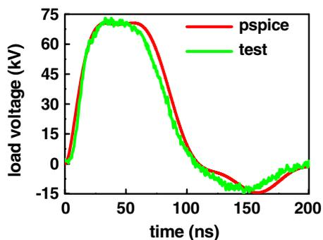
FIG. 11. Recorded and simulated load voltage in a shot with the core, at  $s = 4$ ,  $m = 2$ ,  $R_L \sim 1.6$  Ohm, and  $U_{CH} = \pm 100$  kV. Compared with Fig. 8, the installation of the core reduces the voltage amplitude from  $\sim 77$  kV to  $\sim 70$  kV because of energy loss in the core.
