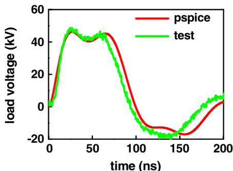
FIG. 13. Recorded and simulated load voltage at  $s = m = 2$ ,  $R_L \sim 1.6$  Ohms, and  $U_{CH} = \pm 100$  kV. At reduced  $s/m$  the pulse becomes double peaked.
