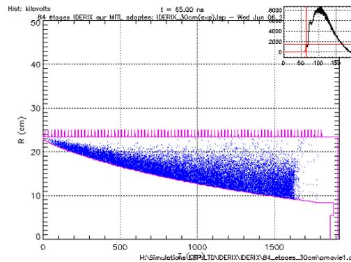
**Figure 9.** View of the electron flow in the IDERIX vacuum line at the time  $t = 65$  ns.
