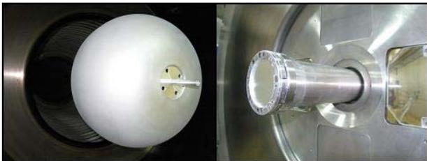
**Figure 12.** Photography of the cathode (on the left) and the anode converter (on the right) of the self magnetic pinch diode
