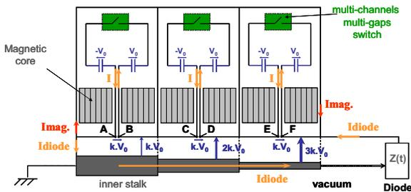
Figure 2. Principle scheme of LTD voltage addition
