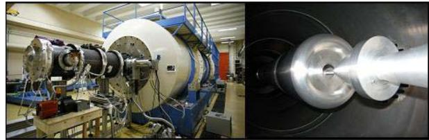
**Figure 13.** Photography of the MITL added to ASTERIX generator (on the left) and of the rod pinch diode (on the right)
