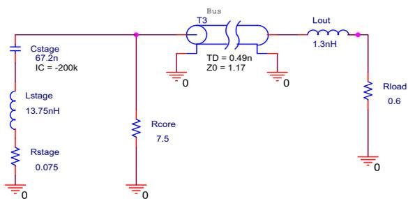
**Figure 5.** Electric circuit used to simulate the super fast LTD stage
