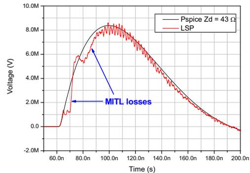
**Figure 10.** Comparison between LSP and Pspice results for the voltage after the last stage
