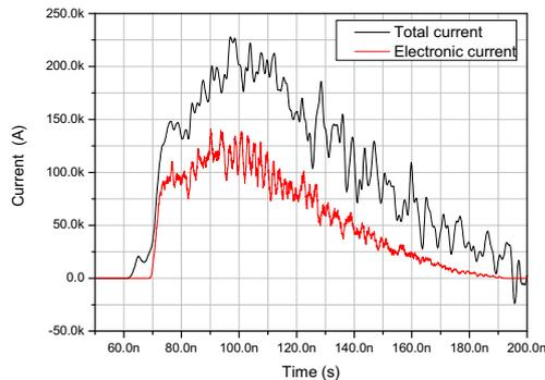
**Figure 11.** LSP results for the total current and electronic current due to the electron flow in the line after the last stage
