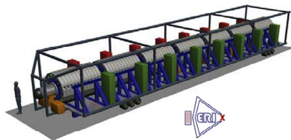
**Figure 1.** Artist view of the flash X-rays machine IDERIX
