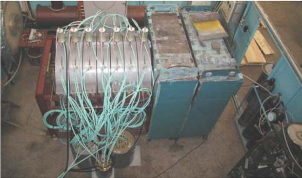
Figure 3. Photography of the SNL 1 MV LTD module
