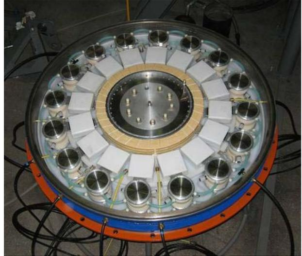
Figure 4. Photography of the first super fast LTD stage
