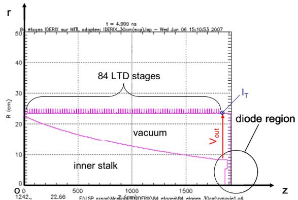
**Figure 8.** LSP geometry to simulate IDERIX
