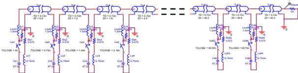
**Figure 7.** Pspice circuit used to simulate the pulsed power generator of IDERIX
