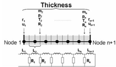
FIGURE 6. Numerical scheme for the MHD routine
