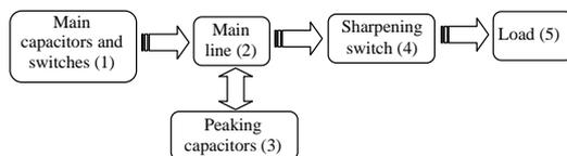
FIGURE 3. Synoptic of the pulser architecture
