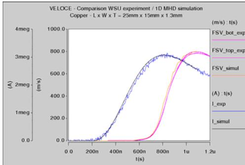
FIGURE 7. Comparison between experiment and simulation - 15mm wide copper load -  $U_0=75\text{kV}$
