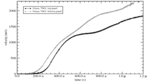
FIGURE 5. Free surface velocities on a 10 mm wide 15mm long copper load with electrodes 1.0mm thick (1.3g) and 1.2mm thick (1.6g) with  $U_0=75\text{kV}$
