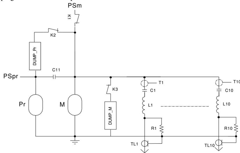
**Figure 2.** Electrical schematics of the capacitor bank module.
