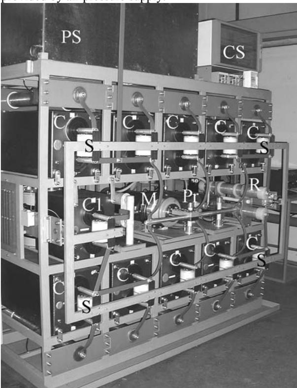
**Figure 3.** Front view of the capacitor bank module.
