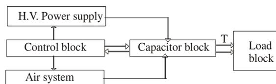
**Figure 1.** Block scheme of the CBM
