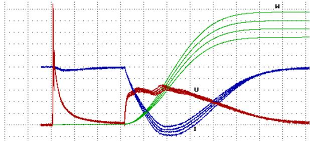
**Figure 4** FL voltage V, current I and energy W waveforms for 21, 22, 23, 24 kV charging voltage (4 kA, 4 kV, 7.5 kJ, 80  $\mu$ s per division).
