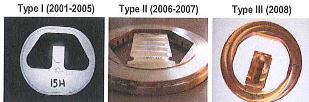
Fig. 6. Evolution of the strip line geometry. Major improvements have been achieved with type III regarding pressure homogeneity.
